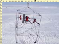
Figure 6: Deployment of the bottom camera
