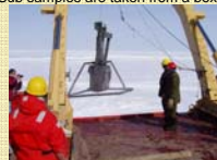
Figure 2: Picture of the box corer deployment
